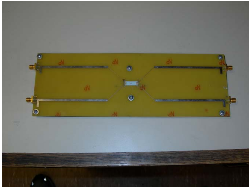
Figure 18: Completed PCB board as tested
