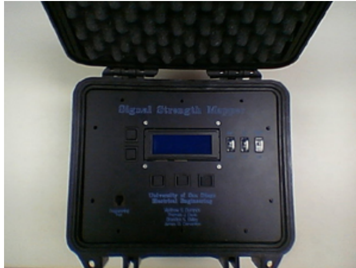
Figure 13: Final Project Aluminum Control Panel and Case
